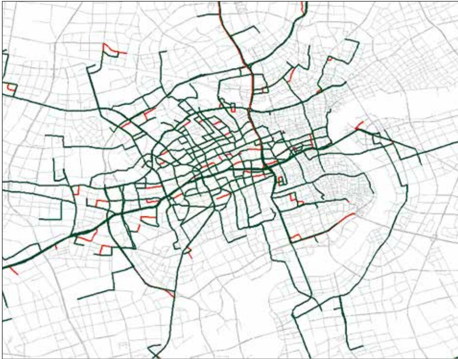
Fig. 3: Map matching results of CRF_L1 (red) overlaid by the ground truth (green) on the road networks of OSM (grey) (Yang 2016)
